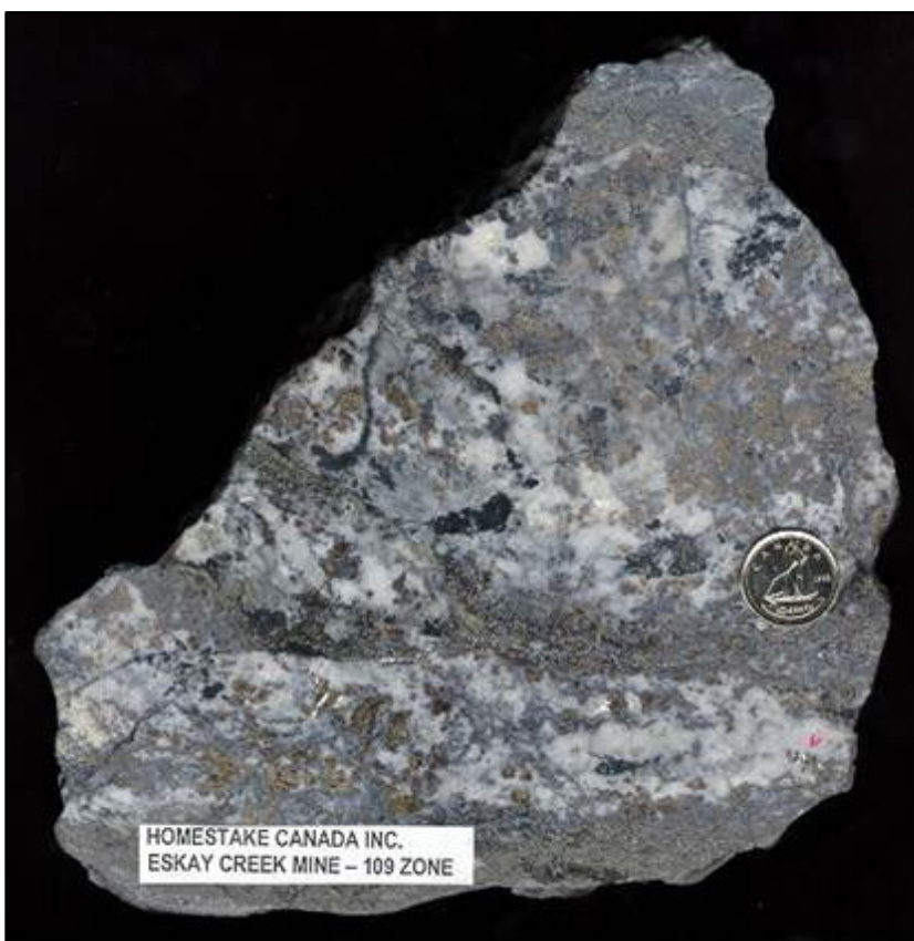
Figure 7-8: 109 Zone - Stockwork veins of quartz-sphalerite-galena-pyrite-gold in the Eskay Rhyolite (Gale et al., 2004).
