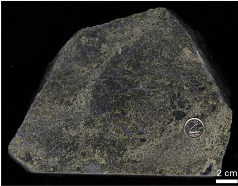
Figure 7-6: NEX Zone - Massive sulphides containing local chalcopyrite within the Contact Mudstone (Gale et al., 2004)
