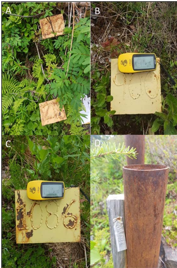
Figure 12-1: Drill hole locations with labelled casing
