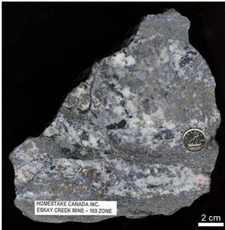
Figure 7-8: 109 Zone - Stockwork veins of quartz-sphalerite-galena-pyrite-gold in the Eskay Rhyolite (Gale et al., 2004).
